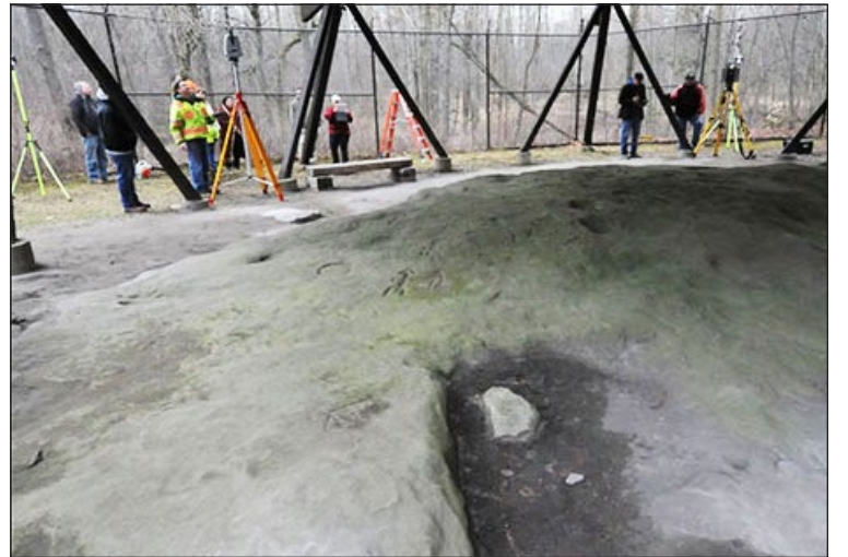
MDOT photo, courtesy of Michigan State Historic Preservation Office The MDOT team at work surveying the Sanilac Petroglyphs using two LiDAR scanners simultaneously.
